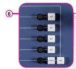
> Settings: allows you to access all of the Orchestra menus and functionalities quickly and easily. The 4 top rotative knobs will allow you to set values, while the last knob will allow to navigate through the interface, to access source or element settings for example.
